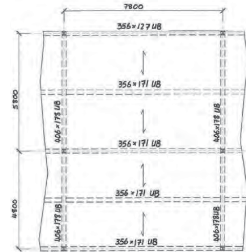
Figure 2: Typical building bay – composite deck option 1
